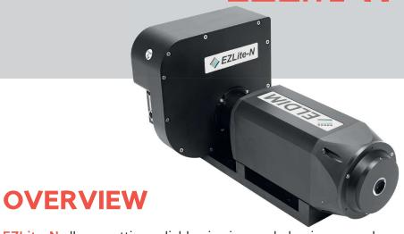
**EZLite-N** allows getting reliable viewing angle luminance and color data. It provides fast and accurate measurements of the full viewing cone with high angular resolution. **EZLite-N** measures a +/-60° viewing angle luminance map in less than 10s.
