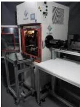
*THOR* systems, full turnkey solutions allowing the analysis of one or more screens simultaneously under temperature stress situation between -40°C & +85°C. Those systems can be used for analyzing several displays in a fully automated way.
