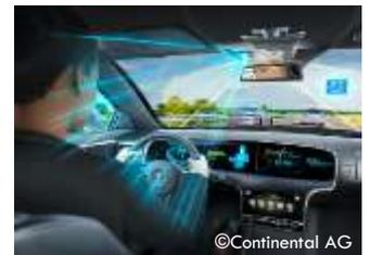
While these two sensor systems both have advantages and disadvantages, infrared sensors allow greater precision in the 3D geometry of the cabin and driver. This makes it easier for a NIR system to scan the driver's face for signs of tiredness or drowsiness.
